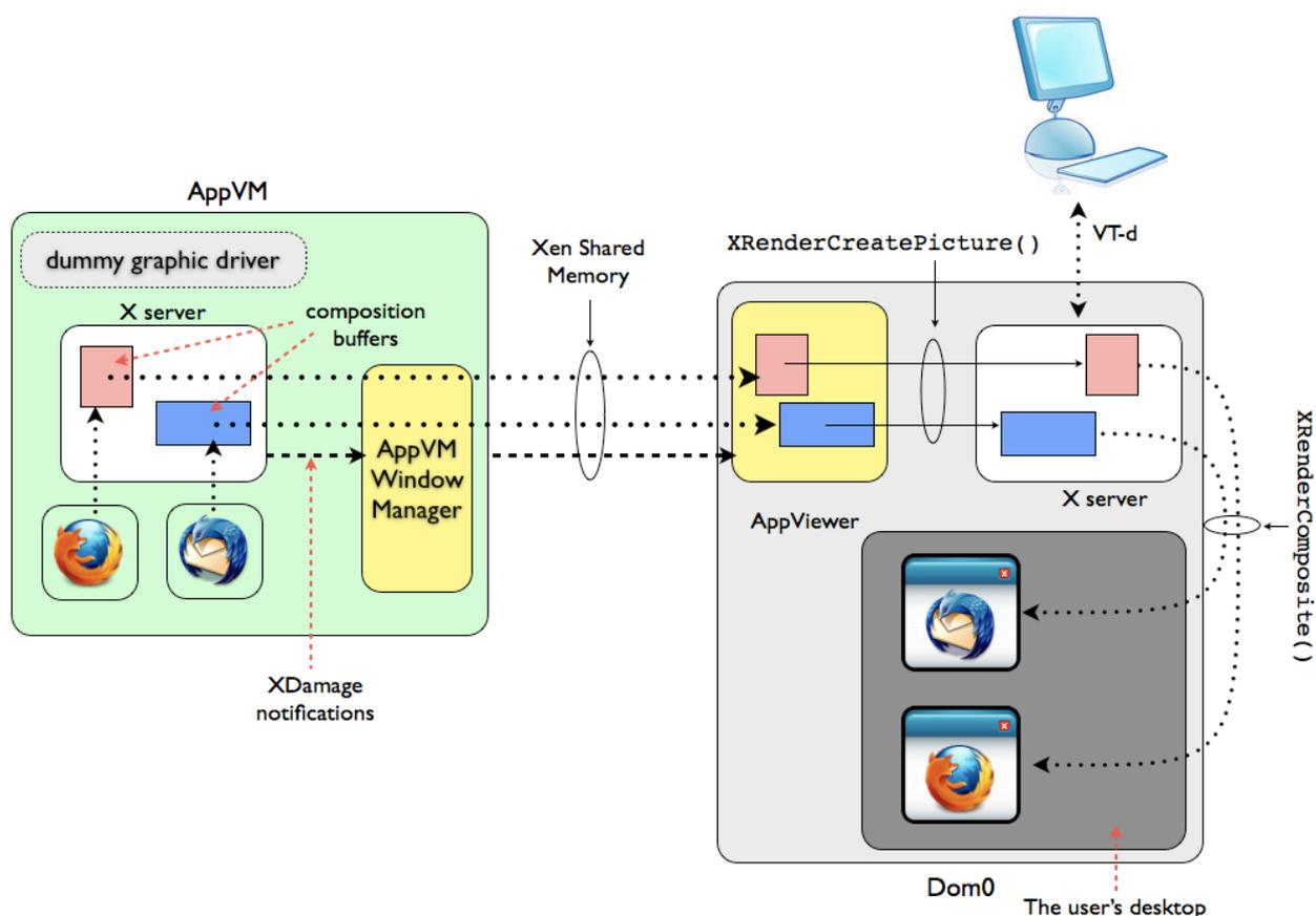
Figure 2. Efficient implementation of AppViewer using composition buffers (requires *XComposite* extension to be enabled in the AppVM's X server).
