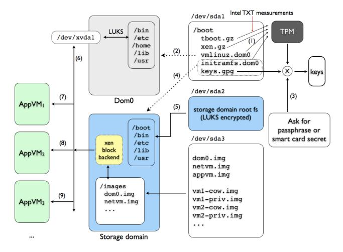
Figure 2. The Qubes OS secure boot process.
